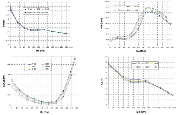
mixtures B80 (increase about 5%). That phenomenon is caused by the big amount of oxygen in methyl esters and what fallows lower demand for oxygen during combustion in engine chamber.
