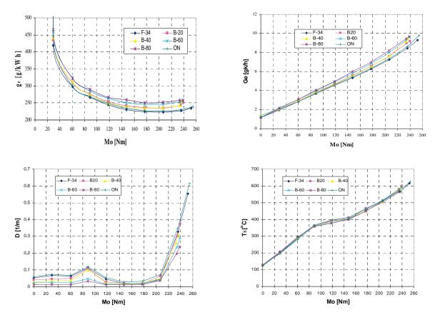
Fig. 6. The weight-bearing characteristics of the engine Renault G9T, n = 1500 rpm, a) the unit consumption of the fuel, b) the hourly consumption of the fuel, c) the fogging the exhaust gas, d) the temperature of exhaust gas before turbocharger
