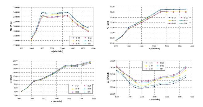
Fig. 2. The external profiles of the engine Renault G9T, a) torque, b) useful power, c) the hourly consumption of the fuel, d) the unit consumption of the fuel
