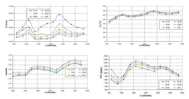
Fig. 3. The external profiles of the engine Renault G9T: a) the fogging the exhaust gases, b) the temperature of exhaust gases behind compressor, c) the coefficient of the excess of the air  $\lambda$ , d) part NOx in the exhaust gas
