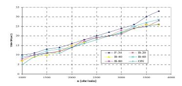
*Fig. 5. The influence of the speed of engine on the increase of the temperature of fuel in the arrangement of the power supply*
