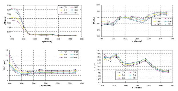
Fig. 4. The external profiles of the engine Renault G9T: a) the part of CO in exhaust gases, b) the part  $O_2$  in exhaust gases, c) the part THC in exhaust gases, d) the part  $CO_2$  in the exhaust gas
